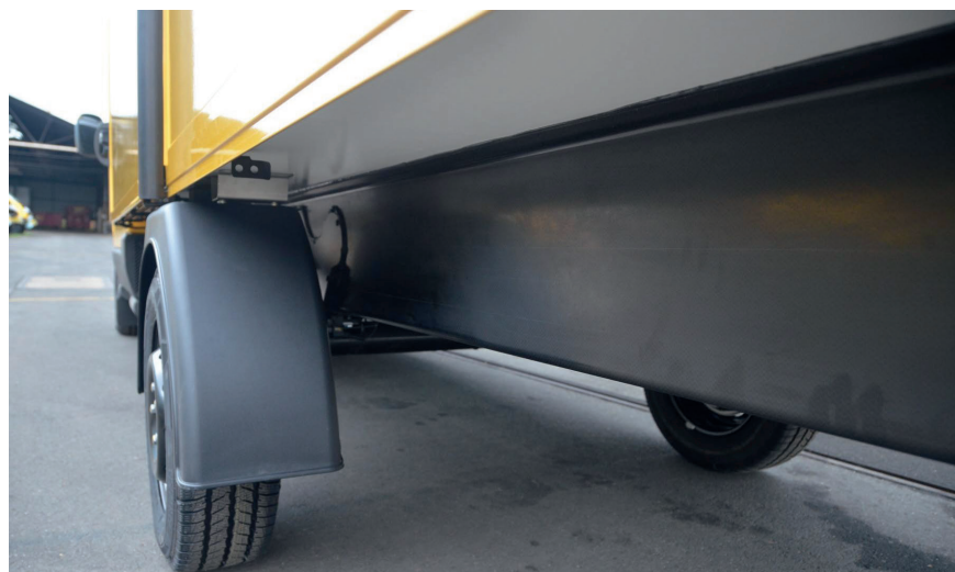
The chassis made from CFRP components are up to 60 % more lightweight than comparable steel designs that are produced at Carbon TT in Buxtehude, Germany. Pultrusion technology from Pultrex is the technical basis of the new production. © Carbon TT
